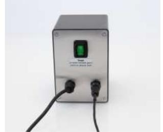
Connect the cable to the external power supply unit and connect the power supply unit with power.
