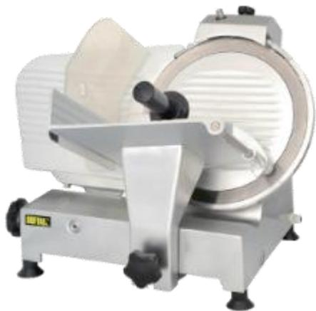
Electric manual meat slicers use a powerful motor to spin a circular blade at high speeds. The user then slides the meat carriage from side to side, accurately cutting the meat to a set thickness. These are sometimes called *gravity slicers* or *self-feeding slicers* as the food carriage is slanted to push the meat against the blade.
